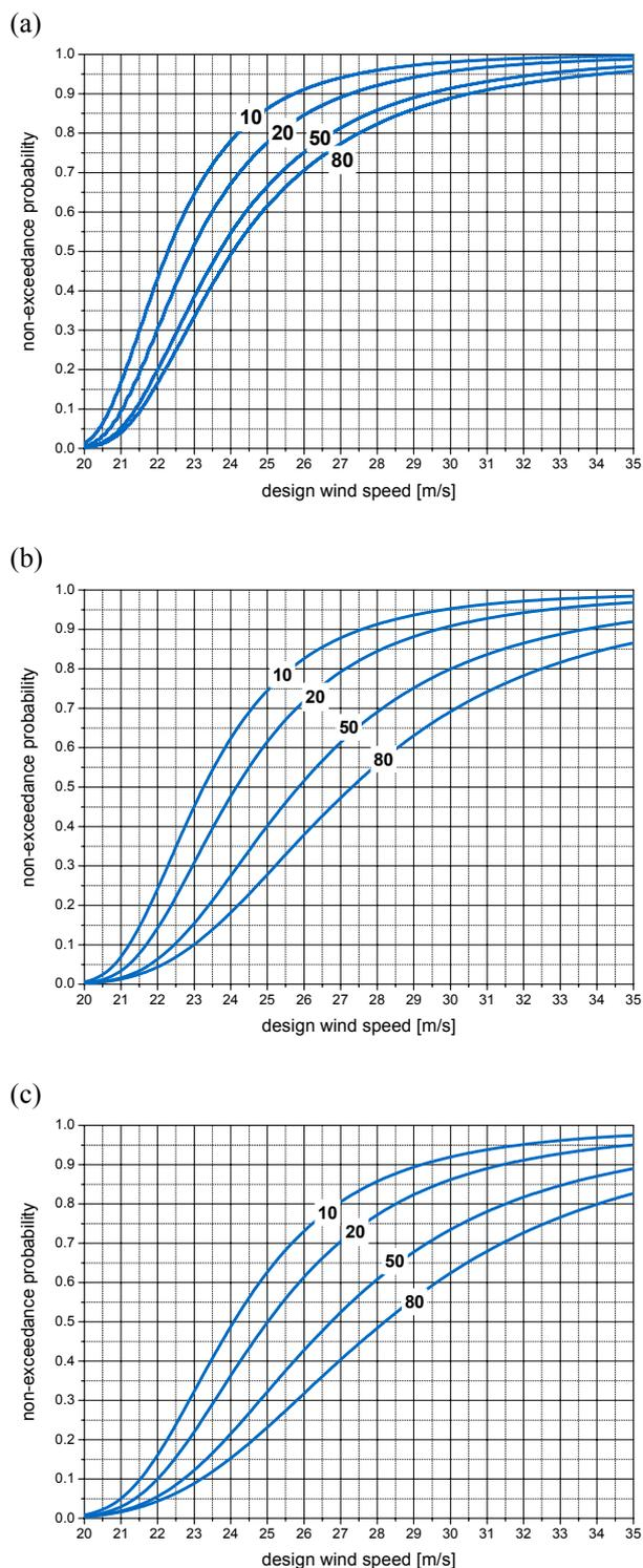
**Fig. 7** Cumulative probability distributions for design wind speed. (a) stationary wind climate, (b) non-stationary wind climate beginning of exposure in 2009, (c) non-stationary wind climate beginning of exposure in 2029.
