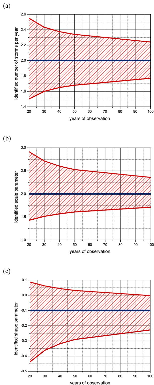
**Fig. 1** Influence of the observation period on the 90%-confidence interval of the statistical parameters of extreme wind climate. (a) number of events per year  $\lambda$ , (b) scale parameter  $s$ , (c) shape factor  $k$
