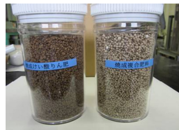
Fig. 14 Pilot-scale kiln system for directly converting incinerated sludge ash to fertilizer by calcination. (A) Rotary kiln for demonstration experiments; (B) Calcined silicate P i fertilizer (left) and calcined mixed fertilizer (right). Photograph courtesy of H. Takano (Taiheiyo Cement Corp.).
