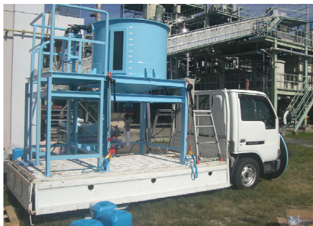
Fig. 12 Mobile pilot-scale plant for the in situ examination and demonstration of P_i recovery from wastewater.
