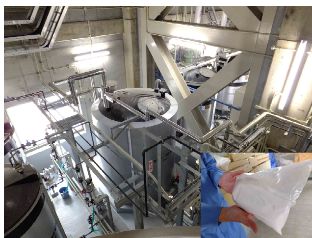
Fig. 4 Full-scale plant for recovering P from sludge incineration ash in Tottori City (inset, recovered product, calcium hydroxyapatite (HAP)). Photograph courtesy of M. Hashimoto (University of Tokyo).
