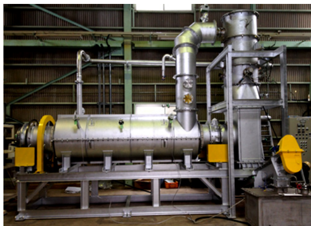
Fig. 13 Pilot-scale plant for carbonization of pig manure in Kobayashi City. Photograph courtesy of K. Ueda (Hitachi Zosen Corp.).
